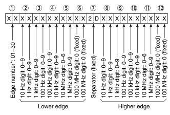
\* Edge number setting is not necessary with command 02.
