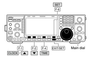
The IC-7600 has a built-in calendar and 24-hour clock (accuracy  $\pm 75$  sec. per month) with daily power ON/OFF timer functions. Before operating these timer functions, set the current date and time.
