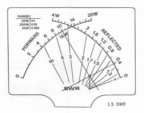
See figure 1. The meter indicates Forwerd  $\,$  power 100W and Reflected Power 4W. At the crossing point of the two meter needles the indication is SWR 1.5.
